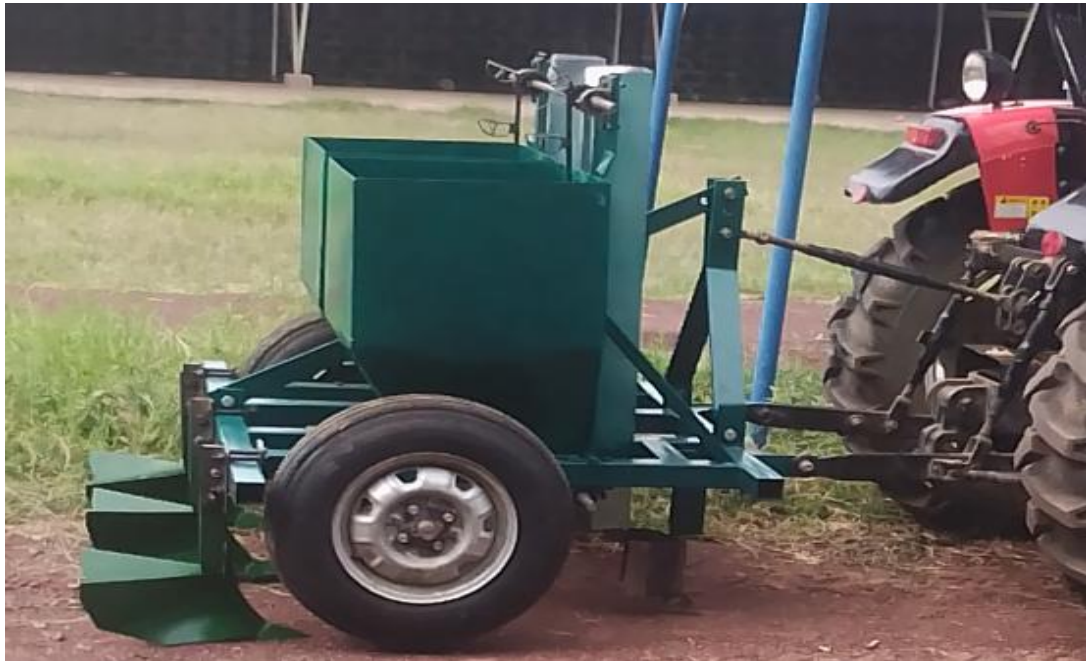
Fig2.3. Fabrication pictures of tractor drawn potato planter
