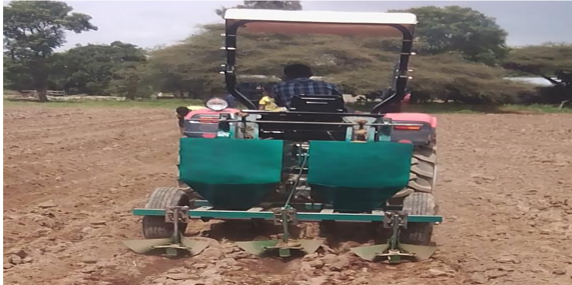
Fig 3.2. Potato Planter under Operation
