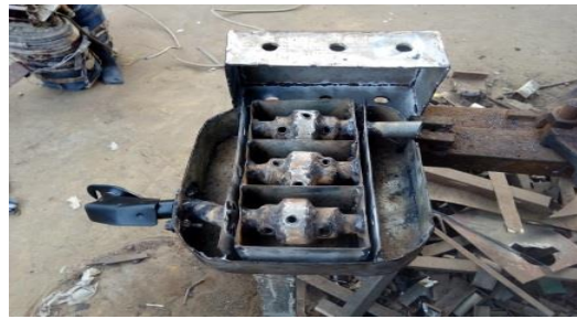
Figure.2 Transverse view of the internals of the newly designed composite muffler
