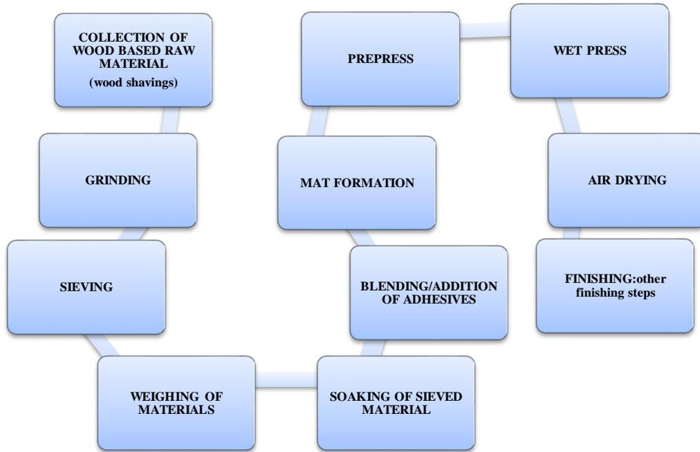
Figure 1: Flow chart of Fiberboard manufacturing
