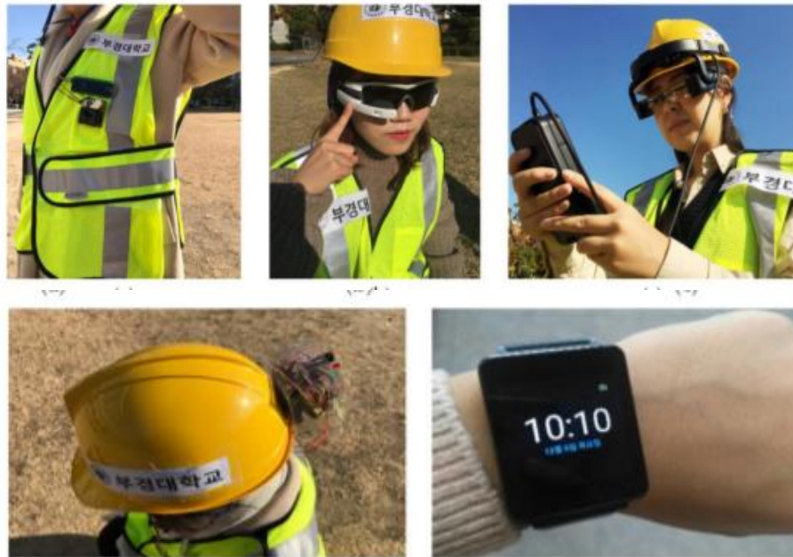
Figure 2: Smart clothing equipped with wearable devices and electronic sensors (Source: (Mardonova & Choi, 2018))
