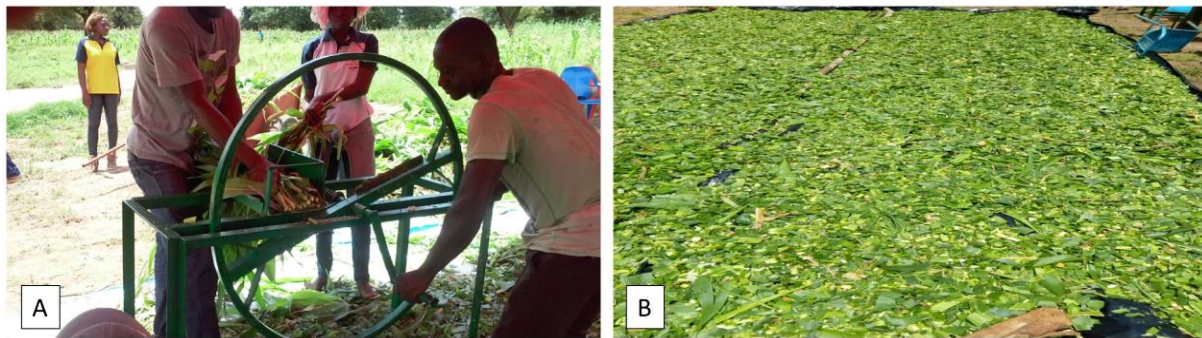
Picture 3: ASMC chopper in use (A) with the chopped forage (B) Millogo (2018).
