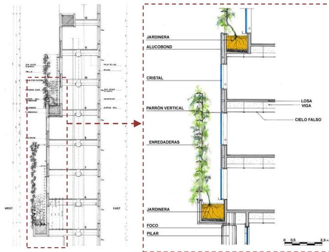
Figure 5: Section Shows the GW location and installation. [10]
