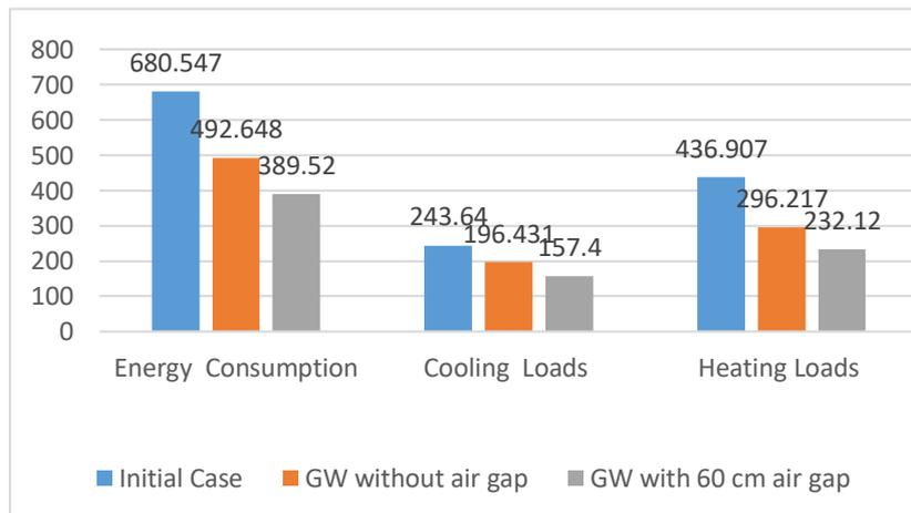
Figure 7: The simulation results for the initial case and the GW installation (with and without airgap).
