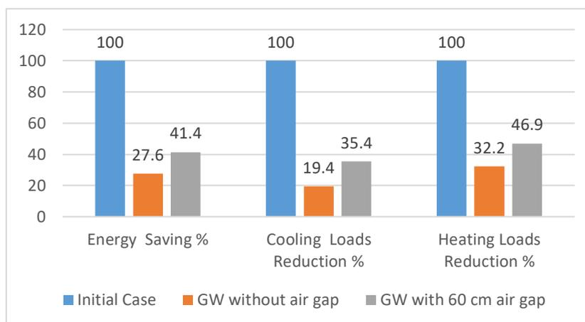
**Figure 8: The Reduction percentage for GW installation (with and without air gap).**
