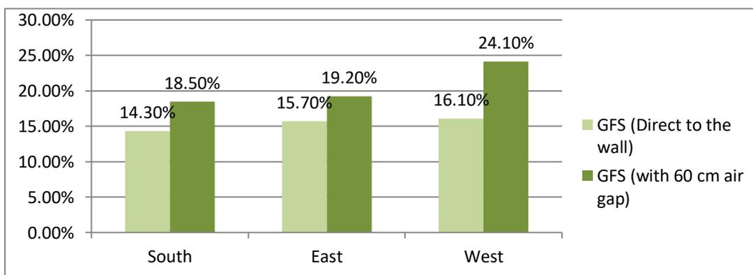
Figure 7: GFS Energy Saving Ratio (both direct and 60 cm air gap)
