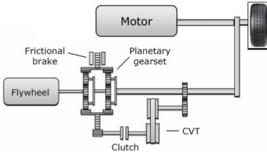
**Figure 3: Simple design Integration of flywheel concept**
