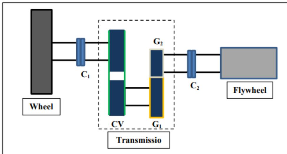
Figure 5: Overall Configuration C: Clutch; G: Gear CV G1 T
