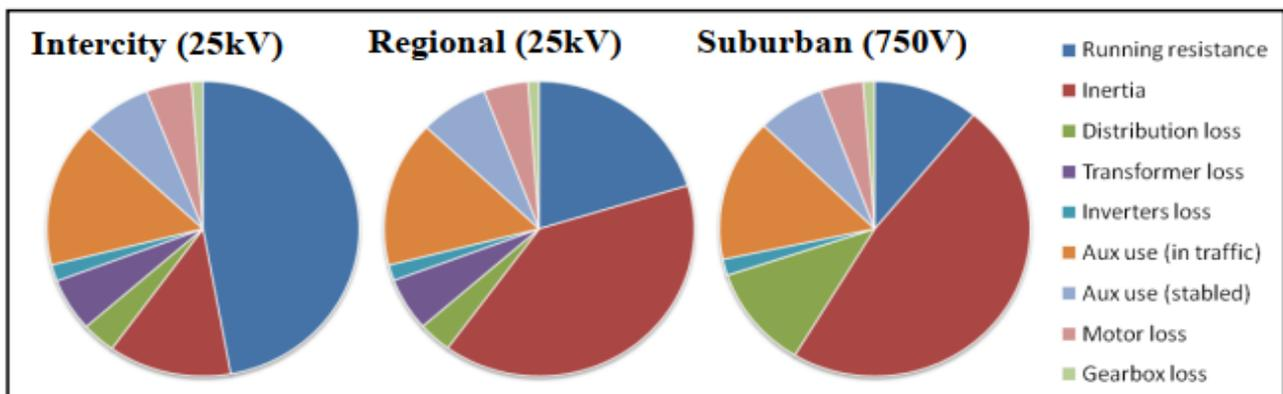
Figure 1: Analysis of energy loss
