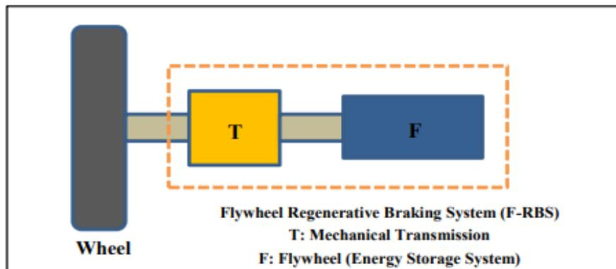
Figure 2: Basic Flywheel Regeneration Model
