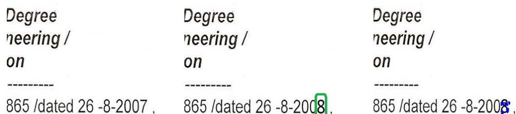
Figure (4): output of error level analysis method. Images from left to right: original, modified text in green rectangle and the output with marked pixels.
