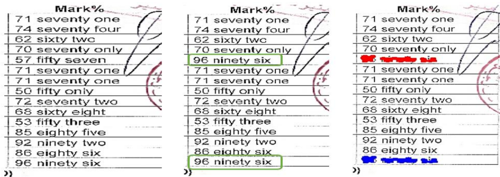
Figure (5): output of copy-move detection method. Images from left to right: original, cloned region in green, output with marked repeated block.
